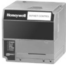
Microprocessor-based integrated full-function primary burner control for automatically fired gas, oil, or combination fuel single burner applications. Programmable Post-Purge. Requires S7800A1142 Display to program post-purge feature.
