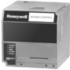
**Integrated full-function primary burner control for gas, oil, or combination fuel single burner applications. Include Programmable Post-Purge and Valve Proving Feature. Requires S7800A1142 Display to program VPS and post-purge features.**
