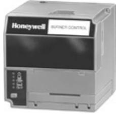
Integrated burner control for automatically fired gas, oil, or combination, single burner atmospheric with fan applications. Has automatic burner sequencing, flame supervising system status indication, system or self-diagnostics, and troubleshooting.
