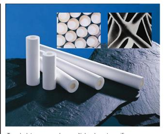
To calculate pressure drop, multiply relevant specific pressure drop by viscosity in centipoise (g.cm $^{-1}$ .s $^{-1}$ ) by flow rate in litres per minute (lpm) [or US gallons per minute (gpm)] divided by cartridge equivalent single lengths (10" multiples). E.g. Clean pressure drop for 20" CP-25 cartridge with water flow of 20lpm (1cP viscosity) = 0.65x1x20/2 = 6.5mbar.
