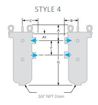
A clearance distance equal to the basket depth must be available above the housing for basket removal. Legs for the Model 4 are optional at an extra cost.
