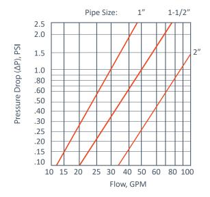
\*Based on housing only. Fluid viscosity, bag filter used, and expected dirt loading should be considered when sizing a filter.
